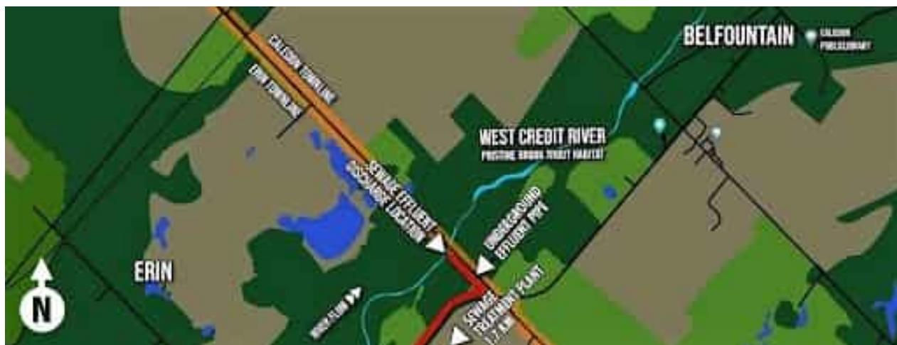
**The facility will have an underground pipe that would bring effluent to the West Credit River.**
